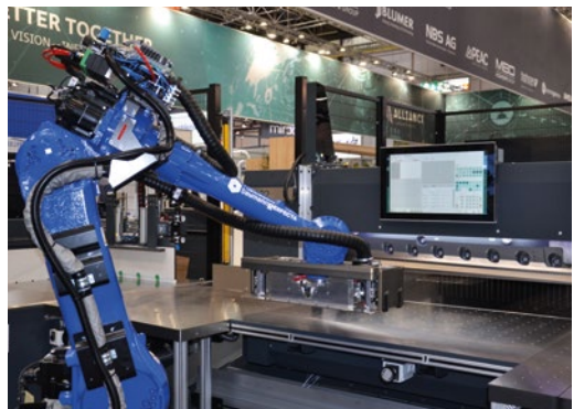
Mannloses Schneiden via Robotic Cutting (RC).
