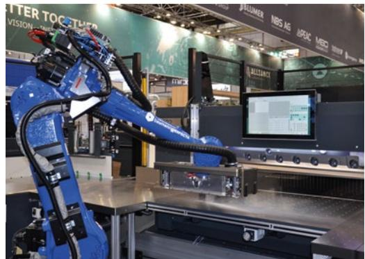
Mannloses Schneiden via Robotic Cutting (RC).
